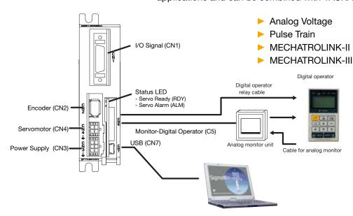
MECHATROLINK-II and III comm. reference doesn't have digital interface. In this case an additional communication port will be embedded.
