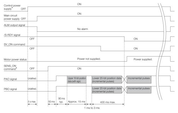
\* When you turn OFF the control power supply, input the SENS\_OFF command.
