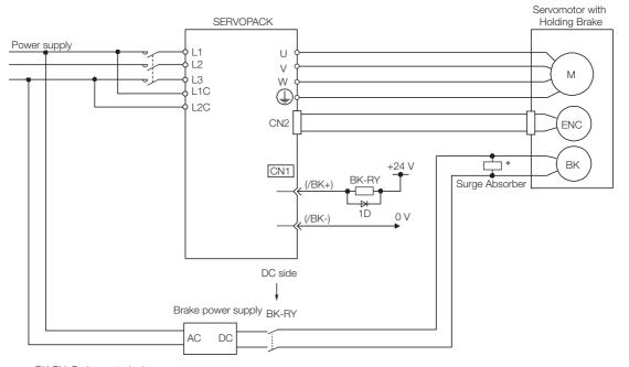
BK-RY: Brake control relay 1D: Flywheel diode
