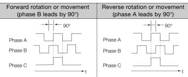
Note: The pulse width of the origin within one encoder rotation depends on the setting of number of encoder output pulses (Pn212) or the encoder output resolution (Pn281). It is the same as the width of phase A. Even for reverse operation (Pn000 =  $n.\square\square\square$ 1), the output phase form is the same as shown above.
