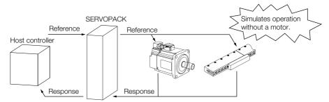
Use  $Pn00C = n.\Box\Box\BoxX$  to enable or disable the test without a motor.
