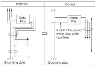
• Connect the Noise Filter ground wire directly to the grounding plate. Do not connect the Noise Filter ground wire to other ground wires.
