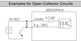
Note: The 24-VDC external power supply capacity must be 50 mA minimum.
