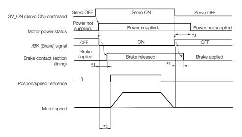
\*1. Rotary Servomotors: The brake delay times for Servomotors with Holding Brakes are given in the following table. The operation delay times in the following table are examples for when the power supply is switched on the DC side. You must evaluate the actual brake delay times on the actual equipment before using the application.
