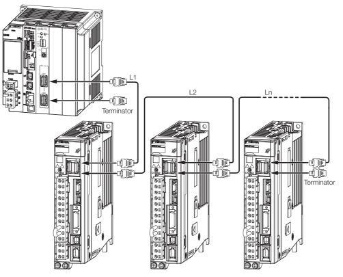
Note: 1. The length of the cable between stations (L1, L2, ... Ln) must be 0.5 m or more.
