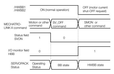
When HWBB Operates While Power Is Supplied to Servomotor
