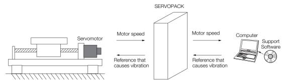
The motor is used to cause machine vibration and then the speed frequency characteristics for the motor torque are measured. The measured frequency characteristics can be used to determine the machine resonance.
