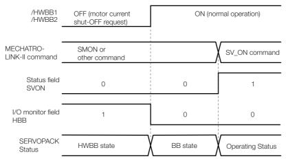
If the /HWBB1 and /HWBB2 signals are OFF and the SV\_ON (Servo ON: 31 hex) command is received, the HWBB state will be maintained even after the /HWBB1 and /HWBB2 signals are turned ON. Send the SV\_OFF (Servo OFF: 32 hex) command to place the SERVOPACK in the BB state and then send the SV\_ON (Servo ON: 31 hex) command.
