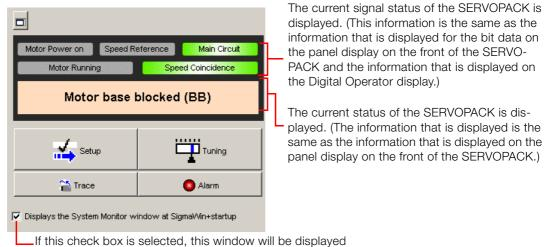
If this check box is selected, this window will be displayed automatically when the SigmaWin+ starts.
