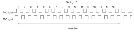
6.5.2 Setting for the Encoder Divided Pulse Output
