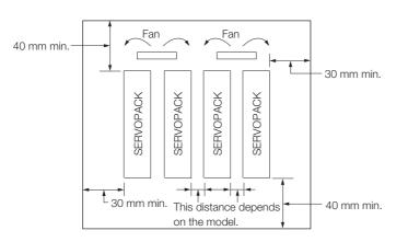
The space required on the right side of a SERVOPACK (when looking at the SERVOPACK from the front) depends on the SERVOPACK models. Refer to the following table.
