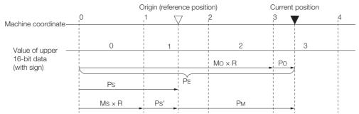
The current position P<sub>M</sub> in the machine coordinate system is calculated as follows:
