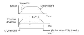
Note: If the parameter is set to a value that is too large, the /COIN signal may be output when the position deviation is low during a low-speed operation. If that occurs, reduce the setting until the signal is no longer output.
