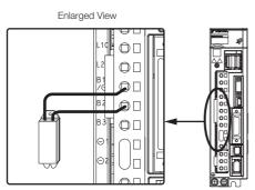
2. Set Pn600 (Regenerative Resistor Capacity) and Pn603 (Regenerative Resistor Resistance).
