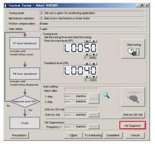
**3.** Click the Import Button or click ▲ and ▼ Button to manually adjust the set frequency. When you click the Import Button, the residual vibration frequency in the motor is read as the set frequency. (The frequency can be read only when the residual vibration frequency is between 1.0 and 100.0.)
