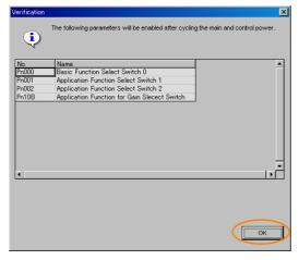
**8.** To enable changes to the settings, turn the power supply to the SERVOPACK OFF and ON again.
