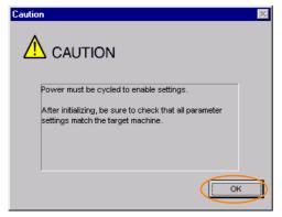
**6.** Turn the power supply to the SERVOPACK OFF and ON again after the parameter settings have been initialized.
