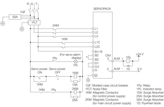
\* You do not have to connect B2 and B3 for the following models: SGD7S-R70A, SGD7S-R90A, SGD7S-1R6A, and SGD7S-2R8A. Do not connect them.
