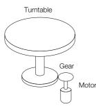
Because the turntable moves in only one direction, the upper limit to the number of revolutions that can be counted by an absolute encoder will eventually be exceeded.
