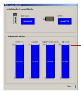
A value of 100% indicates that the SERVOPACK has not yet been used. The percentage decreases as the SERVOPACK is used and reaches 0% when it is time to replace the SERVOPACK.
