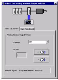
2. Click the Zero Adjustment or Gain Adjustment Tab.
