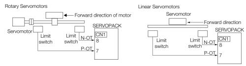
Using the overtravel function is not necessary for rotating applications such as rotary tables and conveyors. No wiring for overtravel input signals is required.
