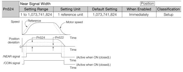
Note: Normally, set Pn524 to a value that is larger than the setting of Pn522 (Positioning Completed Width).
