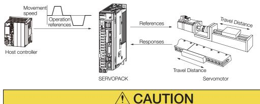
Because autotuning with a host reference adjusts the SERVOPACK during automatic operation, vibration or overshooting may occur. To ensure safety, make sure that you can perform an emergency stop at any time.
