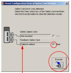
You cannot clear the **Error detected** detection result. Remove the Option Module, or check to see if the Option Module is correctly mounted.
