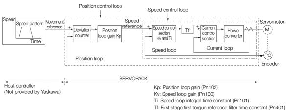
Figure 8.1 Simplified Block Diagram for Position Control
