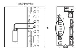
**3.** Set Pn600 (Regenerative Resistor Capacity) and Pn603 (Regenerative Resistor Resistance).
