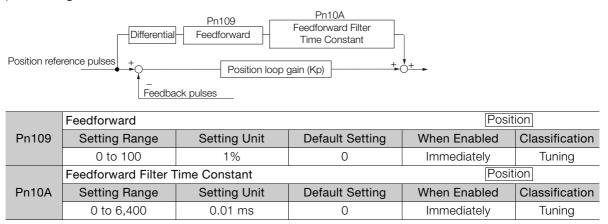
Note: If you set the feedforward value too high, the machine may vibrate. As a guideline, use a setting of 80% or less.
