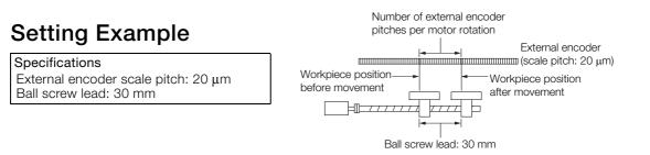
If the external encoder is connected directly to the motor, the setting will be 1,500 (30 mm/0.02 mm = 1,500).
