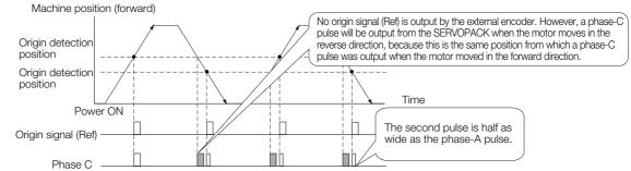
When Passing the First Origin Signal (Ref) in the Reverse Direction and Returning after Turning ON the Power Supply
