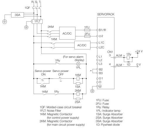
• Wiring Example for DC Power Supply Input: SGD7S-R70A, -1R6A, -2R8A, -3R8A, -5R5A, -7R6A, -120A, -180A, and -200A
