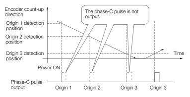
6.5.2 Setting for the Encoder Divided Pulse Output
