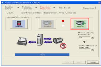
The shaft will rotate in the reverse direction and the measurement will start. After the measurement and data transfer have been completed, the **Forward** Button will be displayed in color.
