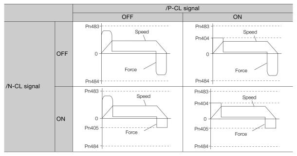
6.7.3 /CLT (Torque Limit Detection) Signal
