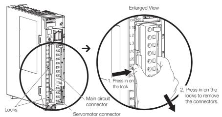
1. Remove the main circuit connector and motor connector from the SERVOPACK.
