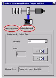
**3.** While watching the analog monitor, use the +1 and -1 Buttons to adjust the offset. There are two channels: CH1 and CH2. If necessary, click the down arrow on the **Channel** Box and select the channel.
