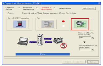
The shaft will rotate in the reverse direction and the measurement will start. After the measurement and data transfer have been completed, the **Forward** Button will be displayed in color.
