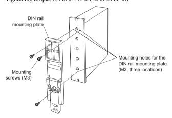
Pull the DIN lever down, engage the upper hooks of the DIN rail mounting plate over the DIN rail, and push the DIN lever until it locks in place.
