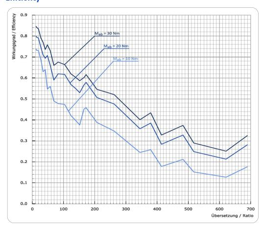
**ZK30** | Two-stage worm helical gear | 03.12.24
