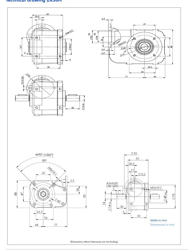
**ZK30** | Two-stage worm helical gear | 03.12.24
