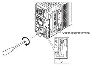
Figure 17 Connect the Ground Wire to the Option
