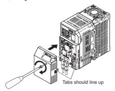
Figure 21 Attach the Option Cover
