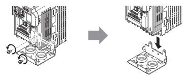
Figure 10 Remove the NEMA Type 1 Conduit Bracket
