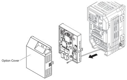
Figure 15 Ground Wire Routing
