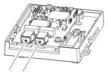
Figure 18 Communication Cable Ports
