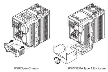
Figure 12 Reattach the Bottom Cover
