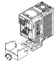
Figure 8 Remove the NEMA Type 1 Terminal Cover (CIMR-V□BA0001F to BA0003F, 2A0001F to 2A0006F)
